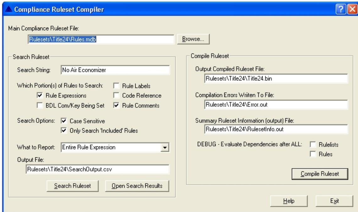
Figure 1: Compliance Ruleset Compiler Application Interface (D2RulCmp.exe)
