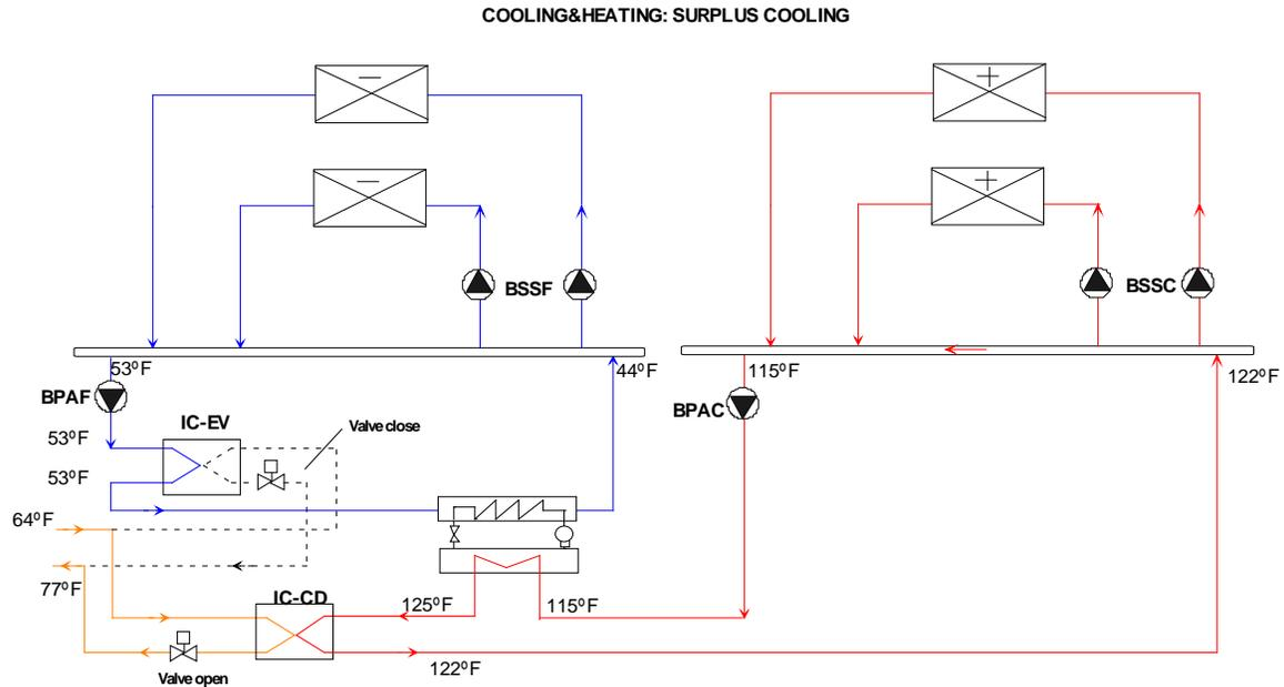
**Figure 33. Loop-to-Loop Heat-Pump
