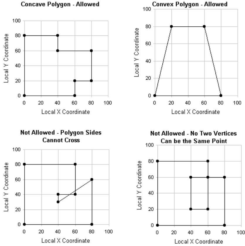
**Figure 11 Example polygons**
