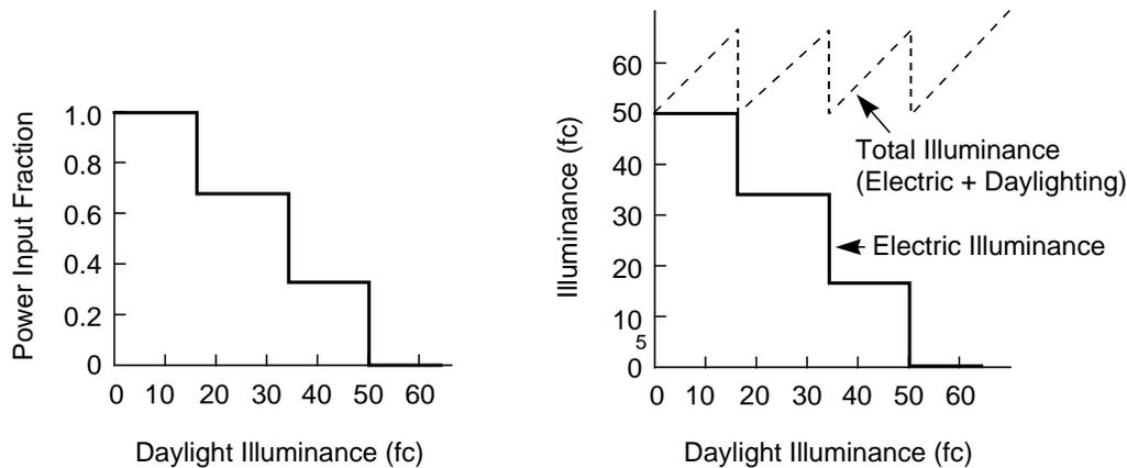
Figure 22 Control action for STEPPED lighting control.
