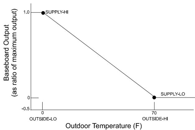
Figure 2 Typical DAY-SCHEDULE-PD:TYPE = RESET-RATIO for baseboard control
