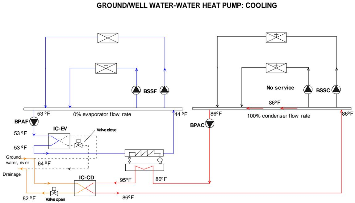
**Figure 31. Loop-to-Loop Heat Pump
