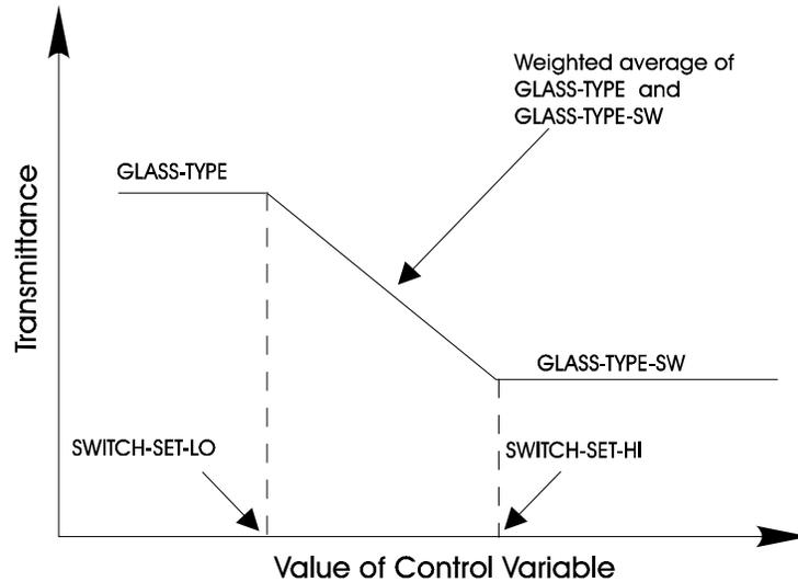
Figure 28 Control Action for Switchable Glazing
