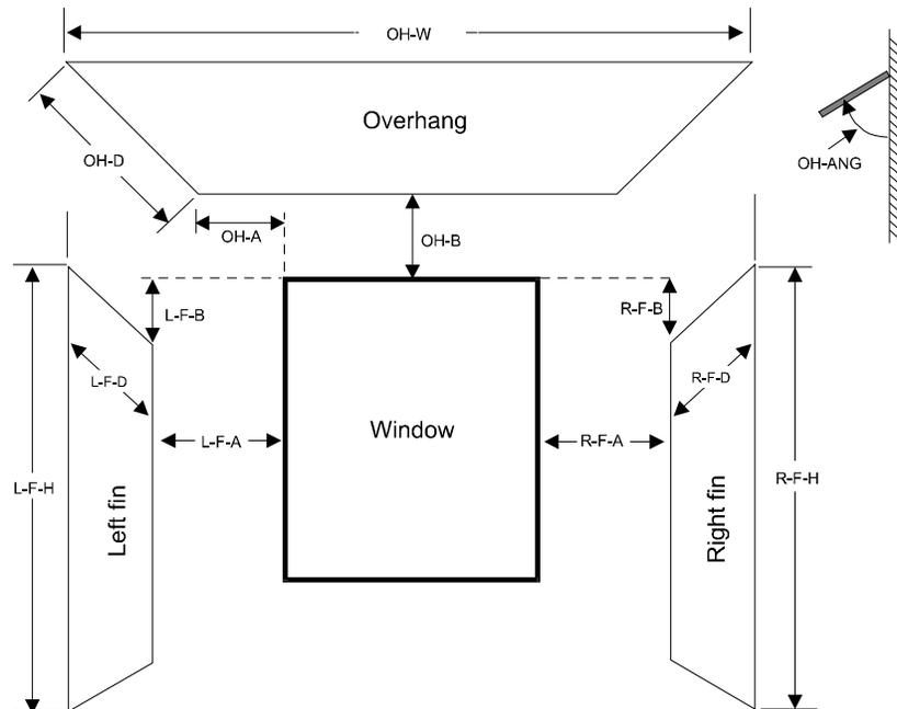
**Figure 26 Positioning of overhang and fins with respect to a window**
