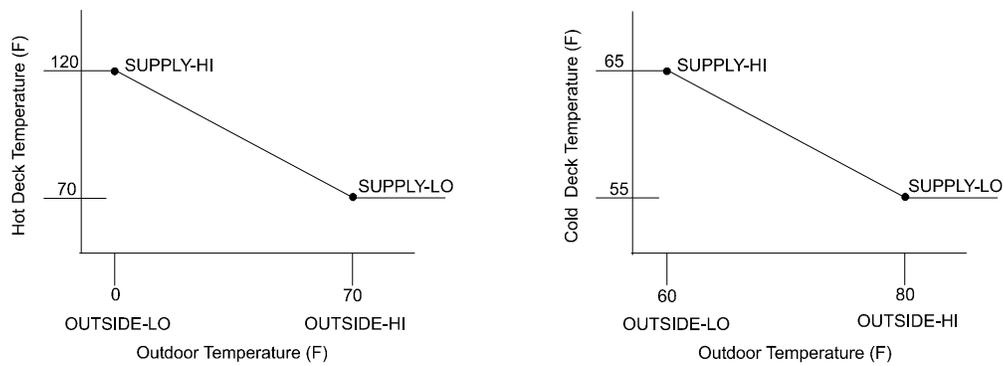
Figure 1 Typical DAY-SCHEDULE-PD:TYPE = RESET-TEMP for deck temperature control
