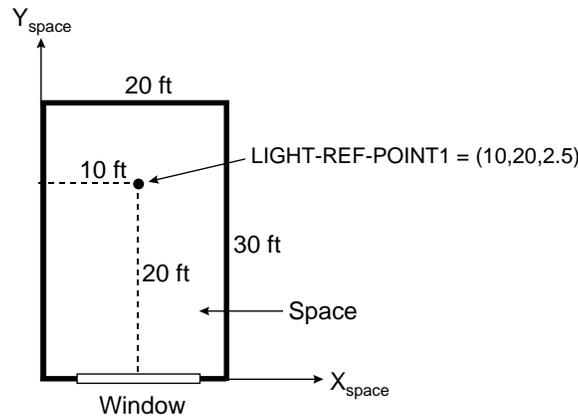
**Figure 18 Plan view of a space.**
