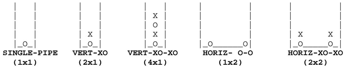
**Figure 35 Pipe arrangements in horizontal wells**
