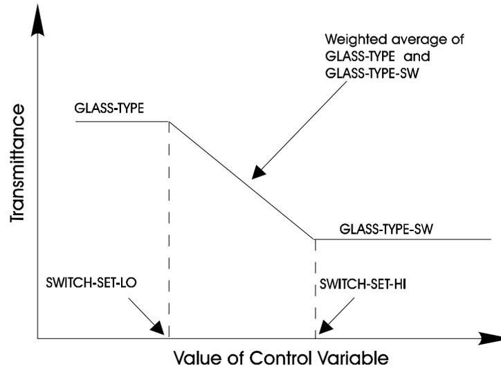
Figure 28 Control Action for Switchable Glazing
