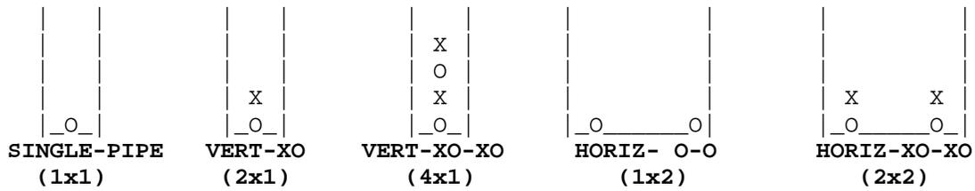
**Figure 35 Pipe arrangements in horizontal wells**
