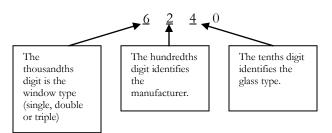
In this set of library entries all window ID's in the 5000 range are single glazed; those in the 6000 range are double glazed and those in the 7000 range are triple glazed. Within each of these window types, glass manufacturer have been assigned a range of ID's. Window ID numbers between 5000 and 5100, and 6000 and 6100 represent generic glazing. Clr/Tint glazings are those glass types that are produced by multiple manufacturers and have nearly the
