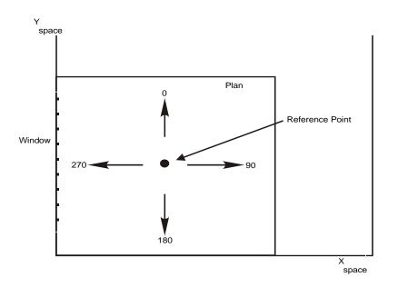
Figure 2 VIEW-AZIMUTH for four occupant view directions. (Daylight glare from the window is greatest when facing window)
