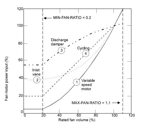
Figure 1 Typical power requirements at part-load operation for four different methods of air flow control. Note that for FAN-CONTROL = CYCLING, MIN-FAN-RATIO is meaningless when the fan is off.
