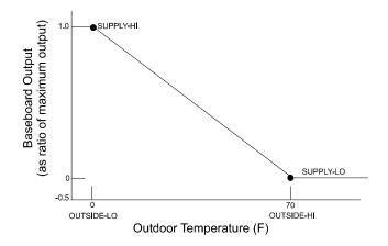
Figure 2 Typical DAY-RESET-SCH FOR baseboard control
