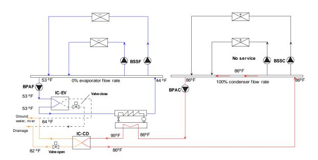
Figure 31. Loop-to-Loop Heat Pump Cooling Only
