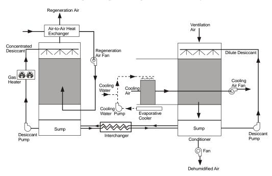
Figure 43 Humidity pump (LIQ-VENT-AIR-1)
