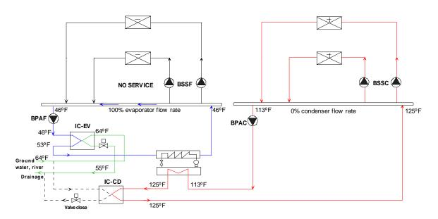
Figure 32. Loop-to-Loop Heat-Pump Heating Only
