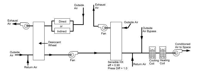
Figure 47 Solid desiccant unit with dehumidifier and heat-exchanger without regeneration preheat, shown integrated with a a sensible cooling system (SOL-VENT-AIR-1 and DESC-CTRL-MODE = 2)
