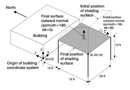
Figure 5 Positioning a shading surface in the building coordinate system
