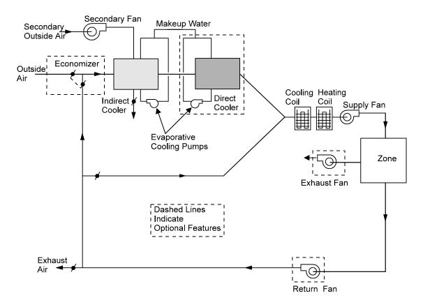
Figure 40 Add-on evaporative cooling unit in which some of the return air passes through the evaporative cooler (EVAP-CL-AIR > MIN-OUTSIDE-AIR), shown integrated with
