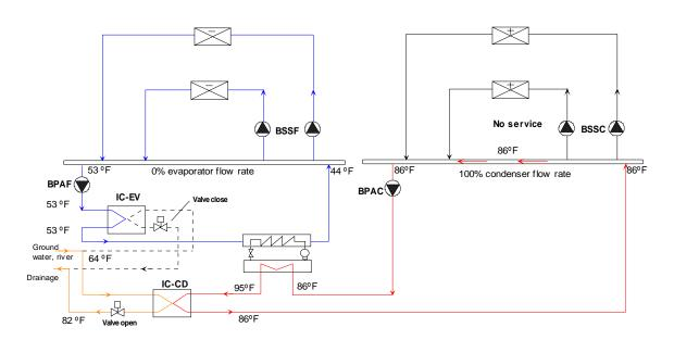
Figure 31. Loop-to-Loop Heat Pump Cooling Only
