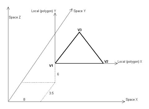
Figure 12 Example 3 triangular wall [The wall has a 90°0 tilt and 180° azimuth, located at X=8, Y=3.5, Z=6 in the space coordinate system. In the coordinate system local to the triangle, the vertex coordinates are V1= (0,0), V2= (20,0) and V3= (10,20)]
