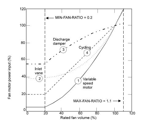
Figure 37 Typical power requirements at part-load operation for four different methods of air flow control. Note that for FAN-CONTROL = CYCLING, MIN-FAN-RATIO is meaningless when the fan is off.
