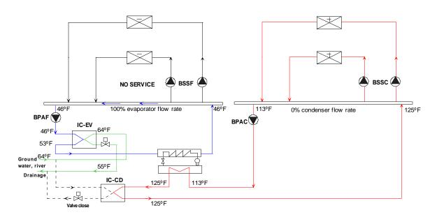
Figure 32. Loop-to-Loop Heat-Pump Heating Only
