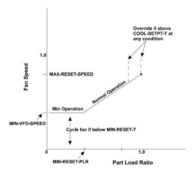
Figure 36 Heat-rejection load reset
