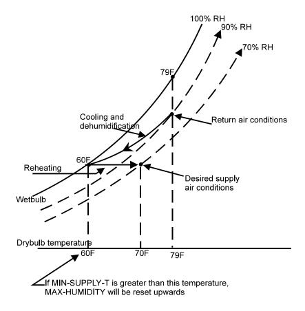
Figure 41 Relationship of MAX-HUMIDITY to MIN-SUPPLY-T
