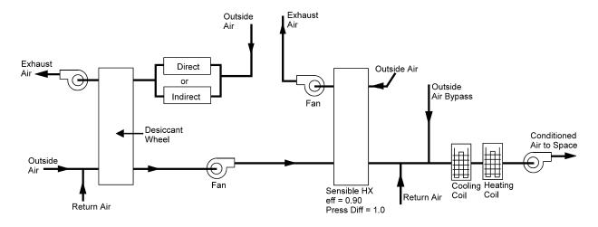
Figure 47 Solid desiccant unit with dehumidifier and heat-exchanger without regeneration preheat, shown integrated with a a sensible cooling system (SOL-VENT-AIR-1 and DESC-CTRL-MODE = 2)
