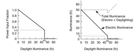
Figure 21 Control action for CONTINUOUS/OFF lighting control. [The lighting set point is 45 fc (482 lux), the minimum power input fraction (MIN-POWER-FRAC) is 0.3, and the minimum electric lighting output fraction (MIN-LIGHT-FRAC) is 0.1]
