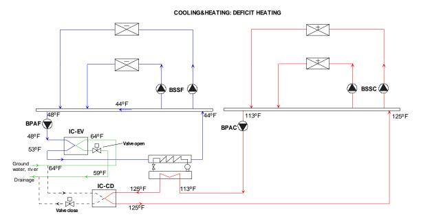
Figure 34. Loop-to-Loop Heat-Pump Heating dominated
