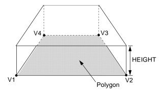
Figure 16 Space extrusion from a polygon
