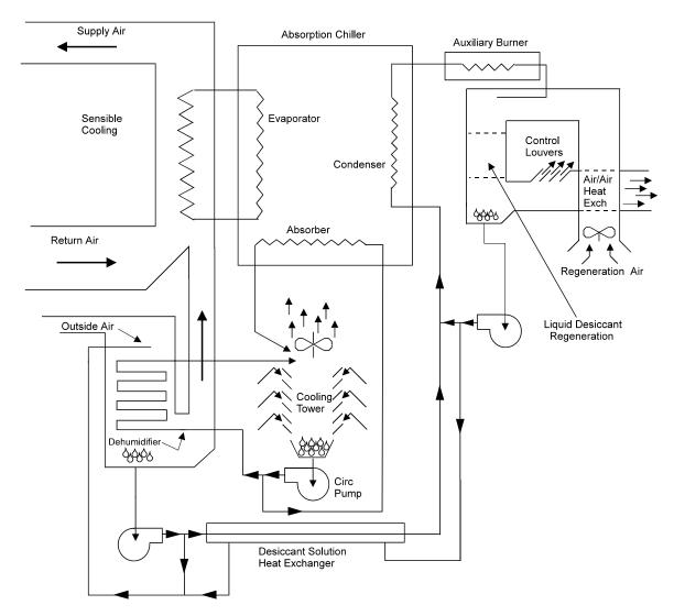
Figure 44 Liquid desiccant dehumdifier unit with gas-fired absorption chiller (LIQ-VENT-AIR-2)
