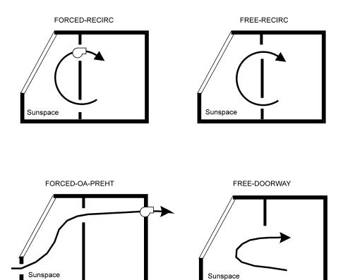
Figure 24 Sunspace INTERIOR-WALL air flow configurations
