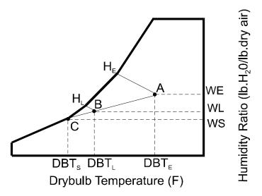
Figure 42 Determining the Coil Bypass Factor
