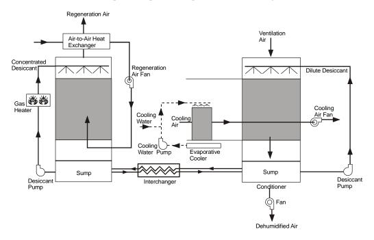
Figure 43 Humidity pump (LIQ-VENT-AIR-1)
