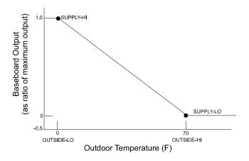
Figure 2 Typical DAY-RESET-SCH FOR baseboard control
