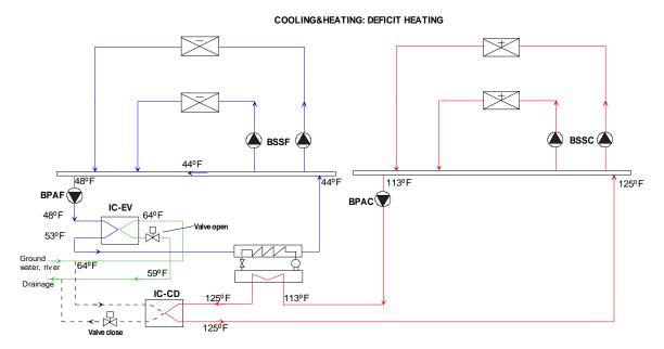
Figure 34. Loop-to-Loop Heat-Pump Heating dominated
