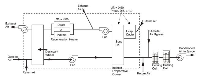
Figure 46 Solid desiccant unit with dehumidifier and heat-exchanger with regeneration preheat, shown integrated with a a sensible cooling system (SOL-VENT-AIR-1 and DESC-CTRL-MODE = 1)
