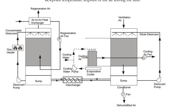
Figure 43 Humidity pump (LIQ-VENT-AIR-1)
