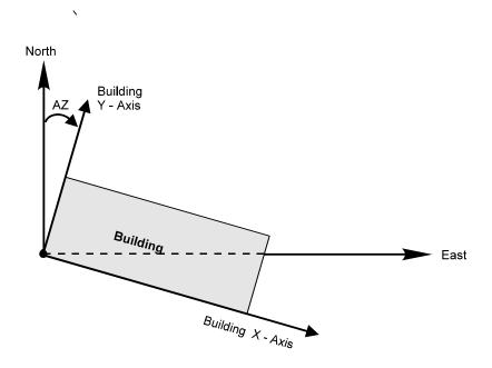
Figure 3 Positioning the building in the reference coordinate system
