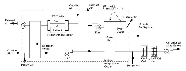
Figure 48 Solid desiccant unit with dehumidifier and indirect evaporative cooler, without regeneration preheat, shown integrated with a sensible cooling system (SOL-VENT-AIR-1 and DESC-CTRL-MODE = 3)
