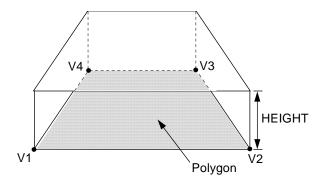
Figure 16 Space extrusion from a polygon
