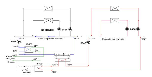
Figure 32. Loop-to-Loop Heat-Pump Heating Only
