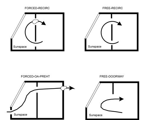
Figure 24 Sunspace INTERIOR-WALL air flow configurations
