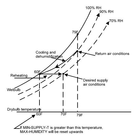
Figure 41 Relationship of MAX-HUMIDITY to MIN-SUPPLY-T
