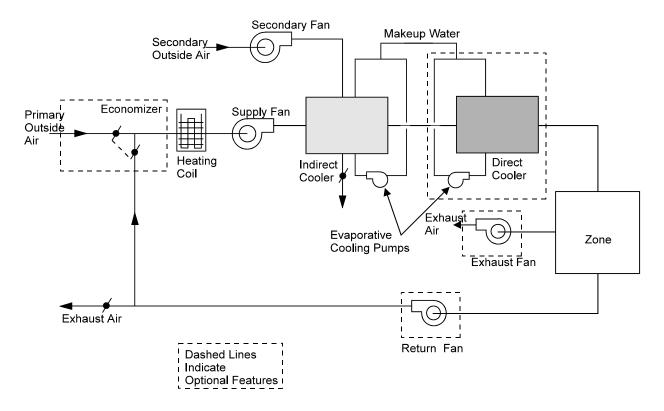
Figure 38 Stand-alone evaporative cooler system (SYSTEM: TYPE = EVAP-COOL)
