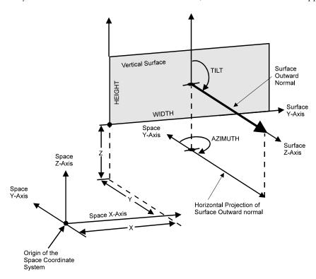
Figure 6 Positioning a wall in the space coordinate system
