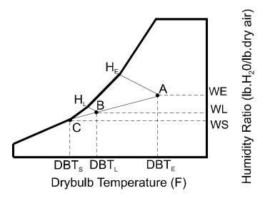
Figure 42 Determining the Coil Bypass Factor
