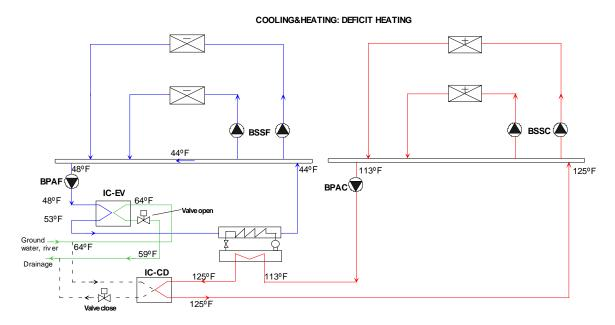
Figure 34. Loop-to-Loop Heat-Pump Heating dominated
