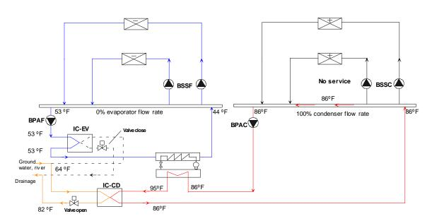
Figure 31. Loop-to-Loop Heat Pump Cooling Only
