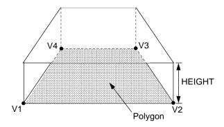
Figure 16 Space extrusion from a polygon
