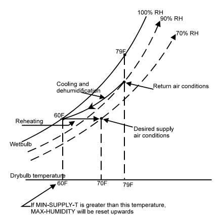
Figure 41 Relationship of MAX-HUMIDITY to COOL-MIN-RESET-T
