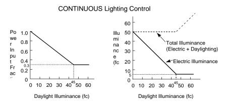
Figure 20 Control action for a lighting system with CONTINUOUS lighting control. [The lighting set point is 45 fc (482 lux), the minimum power input fraction (MIN-POWER-FRAC) is 0.3, and the minimum electric lighting output fraction (MIN-LIGHT-FRAC) is 0.1]
