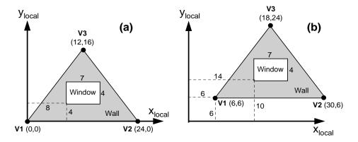
Figure 13 Locating a window or door in a polygonal wall.
