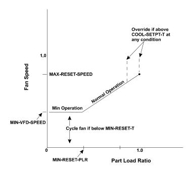
Figure 36 Heat-rejection load reset
