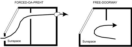
Figure 24 Sunspace INTERIOR-WALL air flow configurations
