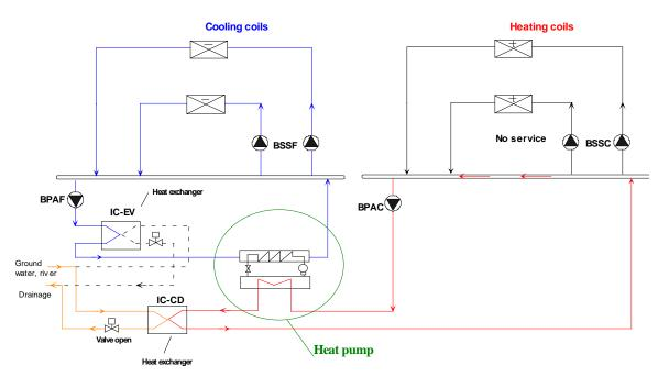
Figure 30. Loop-to-Loop Heat Pump
