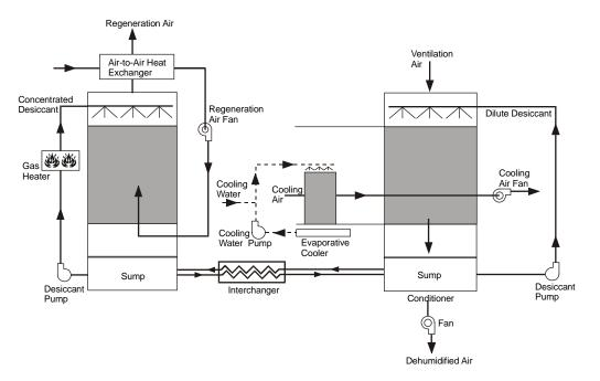
Figure 43 Humidity pump (LIQ-VENT-AIR-1)
