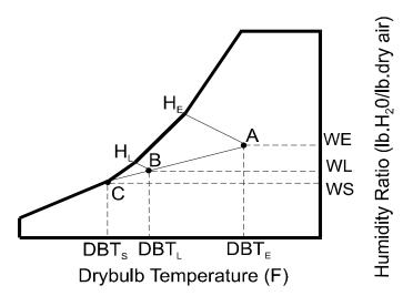
Figure 42 Determining the Coil Bypass Factor
