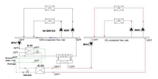
Figure 32. Loop-to-Loop Heat-Pump Heating Only
