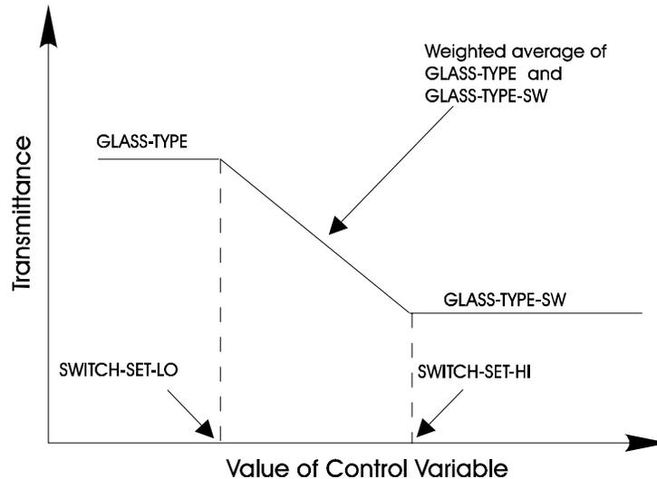
**Figure 28 Control Action for Switchable Glazing**
