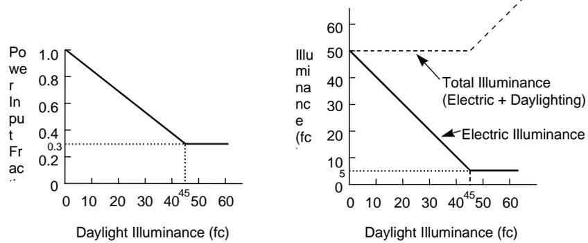
Figure 20 Control action for a lighting system with CONTINUOUS lighting control.
