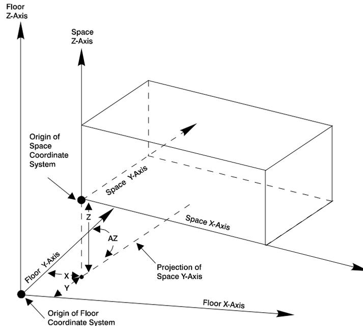
**Figure 15 Positioning the origin of the space coordinate system.**
