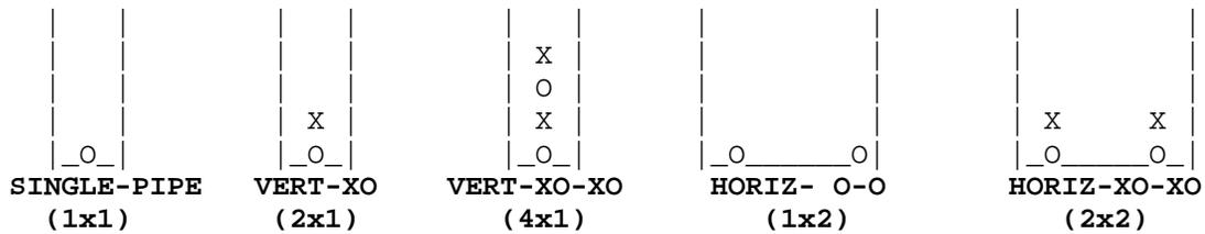
**Figure 35 Pipe arrangements in horizontal wells**
