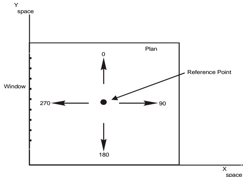
Figure 2 VIEW-AZIMUTH for four occupant view directions.
