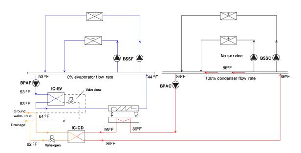
Figure 31. Loop-to-Loop Heat Pump Cooling Only
