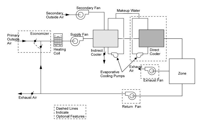
Figure 38 Stand-alone evaporative cooler system (SYSTEM: TYPE = EVAP-COOL)
