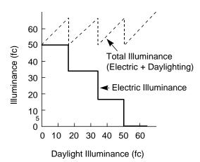
Figure 22 Control action for STEPPED lighting control. [The lighting set point is 50 fc (538 lux) and the number of steps (LIGHT-CTRL-STEPS) is 3]
