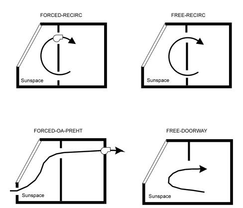
Figure 24 Sunspace INTERIOR-WALL air flow configurations
