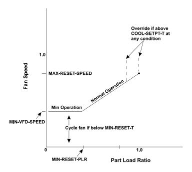
Figure 36 Heat-rejection load reset
