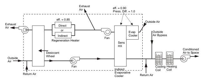
Figure 46 Solid desiccant unit with dehumidifier and heat-exchanger with regeneration preheat, shown integrated with a a sensible cooling system (SOL-VENT-AIR-1 and DESC-CTRL-MODE = 1)
