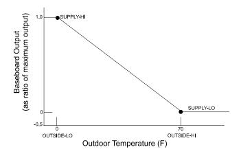
Figure 2 Typical DAY-RESET-SCH FOR baseboard control
