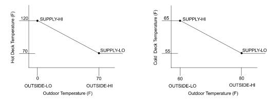
Figure 1 Typical DAY-RESET-SCH for deck temperature control
