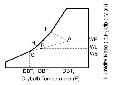
Figure 42 Determining the Coil Bypass Factor
