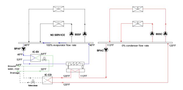
Figure 32. Loop-to-Loop Heat-Pump Heating Only
