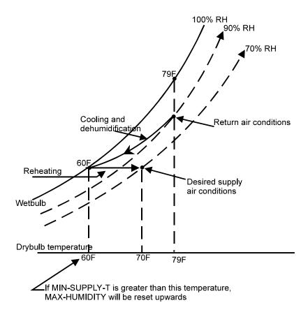
Figure 41 Relationship of MAX-HUMIDITY to MIN-SUPPLY-T
