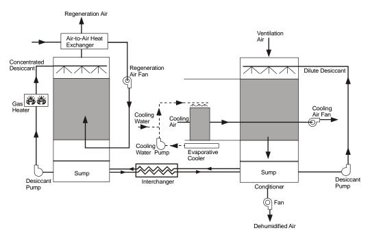
Figure 43 Humidity pump (LIQ-VENT-AIR-1)
