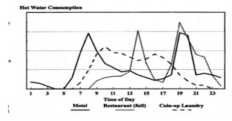
Figure 2. Hot Water Use Profile in Motels, Restaurants, and Commercial Laundries
