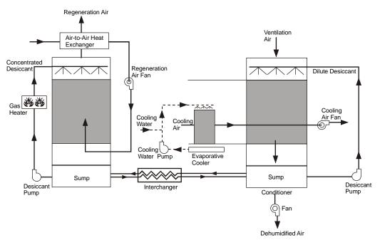
Figure 43 Humidity pump (LIQ-VENT-AIR-1)
