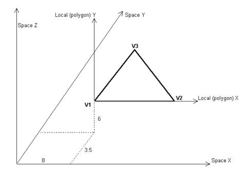
Figure 12 Example 3 triangular wall [The wall has a 90°0 tilt and 180° azimuth, located at X=8, Y=3.5, Z=6 in the space coordinate system. In the coordinate system local to the triangle, the vertex coordinates are V1= (0,0), V2= (20,0) and V3= (10,20)]
