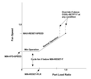
Figure 36 Heat-rejection load reset
