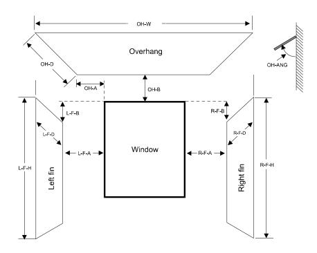
Figure 26 Positioning of overhang and fins with respect to a window (The values in this figure are all positive. If the value of L-F-B is input as a negative, the left fin will originate at a point above the top edge of the window; similarly for R-F-B. If OH-A is input as negative, the overhang will originate to the right of the left side of the window)
