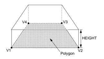
Figure 16 Space extrusion from a polygon
