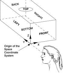
Figure 14 The faces of a BOX in the space coordinate system
