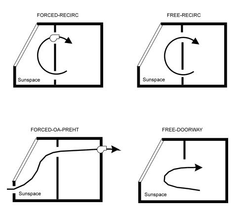
Figure 24 Sunspace INTERIOR-WALL air flow configurations
