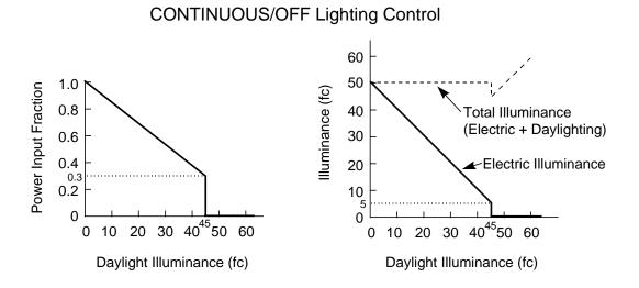
Figure 21 Control action for CONTINUOUS/OFF lighting control. [The lighting set point is 45 fc (482 lux), the minimum power input fraction (MIN-POWER-FRAC) is 0.3, and the minimum electric lighting output fraction (MIN-LIGHT-FRAC) is 0.1]
