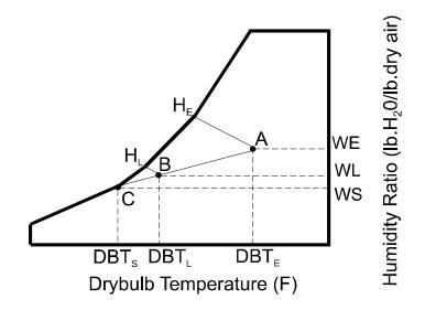
Figure 42 Determining the Coil Bypass Factor
